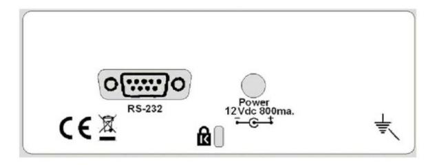
The rear panel has connectors for RS-232 serial and a power input socket. Required power input is a low-voltage external supply, 12VDC @ 800mA.
