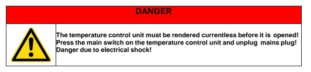
Repair leaks in the temperature control circuit (device, connecting lines, etc.) immediately.
