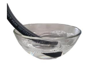
For even easier assembly, use soapy water as lubricant. Simply dip the end of the hose in the soapy water beforehand, and dry off the outer surface of the hose before assembly
