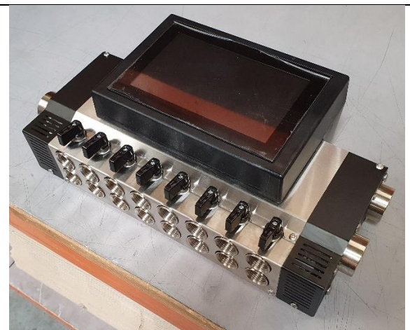
Incomplete 8 zone manifold
